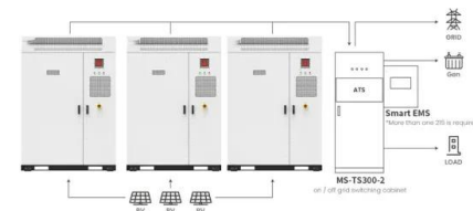
Application scenarios of energy storage battery products
